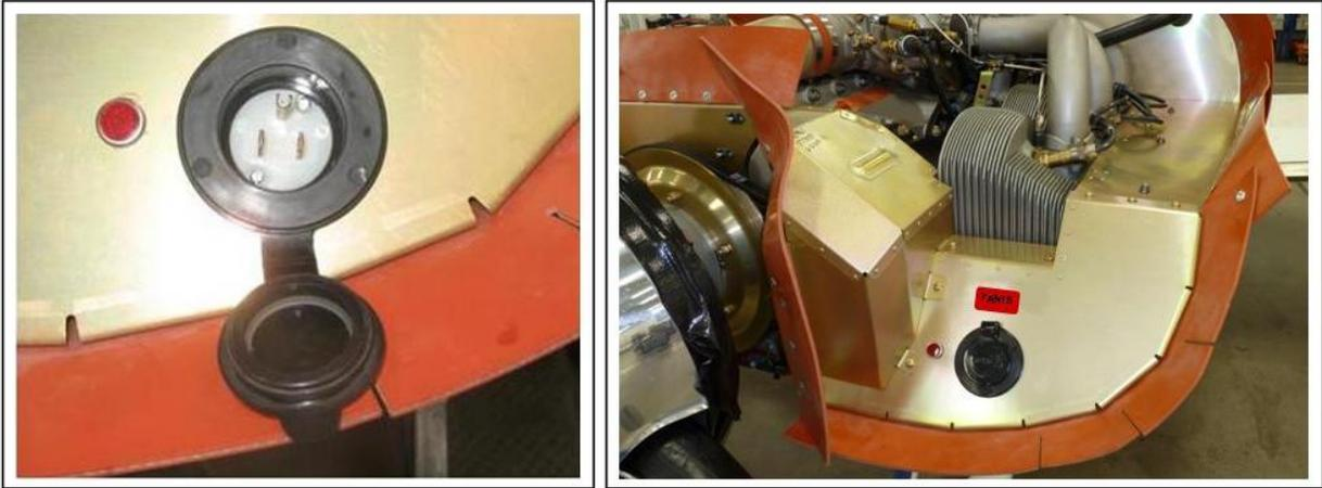
**Figure 2** - SR22/SR22T Shore power plug located in left front engine baffle. Plug for the SR20 (not shown), is located in same area on horizontal surface of baffle.
